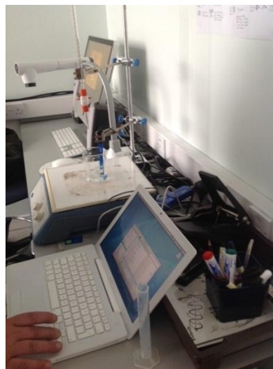
Figure 24. Data loggers used for experiments in a) colour saturation in a chemical reaction using a colour wavelength data logger and b) naturalisation of an acid with alkaline using a PH probe, both attached to data collection software
