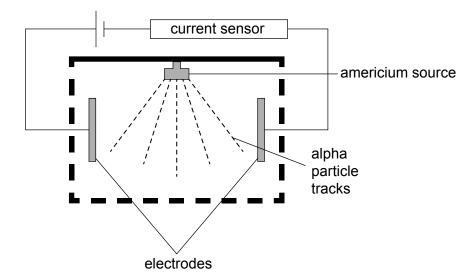
Americium-241 emits alpha particles that ionize the air in the chamber. Each ionization forms one positive ion and one electron; these are called an ion pair. The electrons and the positive ions move towards the electrodes and the sensor detects a current in the air.
